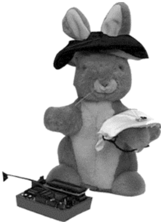
Figure 1: interactive programmable stuffed rabbit and Handy Board (microcontroller)
