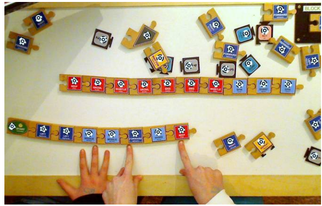
Figure 9. An example screen shot from a program created in the tangible condition. The digital photograph has been cropped for clarity. The field of view of the digital camera includes the entire programming surface.
