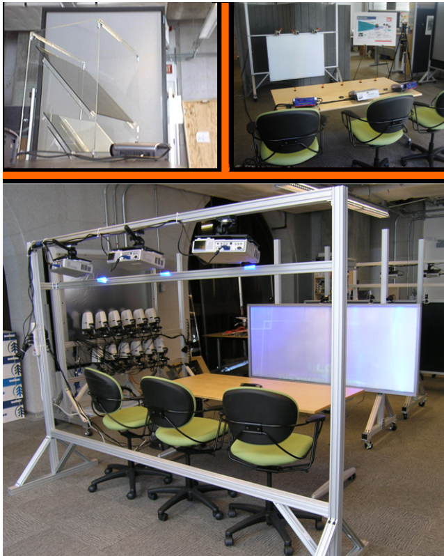
Figure 4. This figure shows the several iterations of MultiView's design. MultiView started as a video tunnel setup with a retroreflective screen (upper left). The video tunnel was abandoned for a front projected directional screen (upper right). The latest iteration includes a larger screen, higher precision optics, short throw projectors, and high resolutions cameras.
