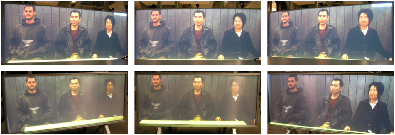
Figure 3. Three remote participants are gazing at viewing position 1 (see Figure 2). Column 1 is the view from position 1, column 2, position 2, and column 3, position 3. The top row is what is seen from the respective positions with non-directional video conferencing and demonstrates perspective invariance. The bottom row is what is seen using MultiView and shows appropriately changing perspectives.
